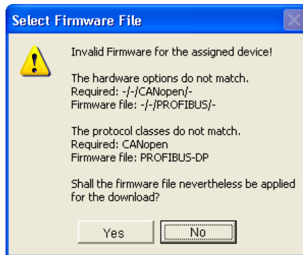
Figure 17: Request Select firmware file - Example Invalid Firmware
