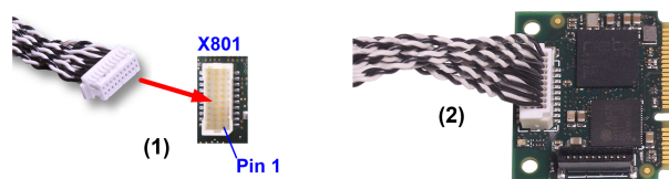
Figure 4: Plug the cable into the cable connector Ethernet on the basic card, example CIFX HPCI90
